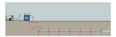
The 33kHz, CF or 131kHz Signal Generator/ Transmitter signal is applied using the 'Direct Connection to a metal pipe' method as shown in the Locator Instruction Manual. Connect the red Direct Connection Lead to the red terminal of the Plastic Pipe Tracer/ Flexible Tracer. Connect the black lead to the Earth Stake. Leave the other terminal of the Plastic Pipe Tracer/ Flexible Tracer unconnected.
