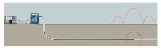
A 33kHz or CF Signal Generator/ Transmitter signal is applied by connecting the red Direct Connection Lead to the red terminal on the Tracer and the black Earth Lead to the other terminal. As the second connection is made a change of pitch should be heard from the Signal Generator/ Transmitter signal indicating successful connection.
