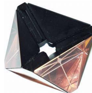
Figure 5 – Six triple-prism glass assembly.
