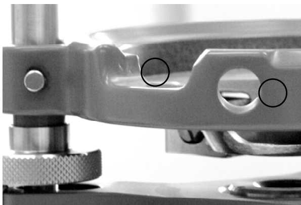
Figure 6 - Detail view of WILD GDF6 tribrach
