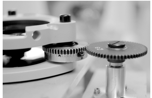
Figure 13 - Tribrach lifetime test setup
