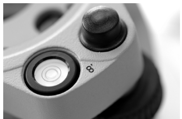
Figure 4 - Detail view of the GDF121 circular bubble
