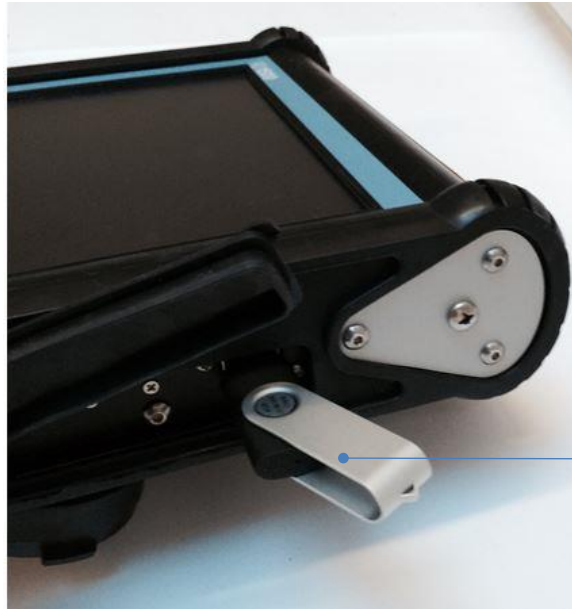
Figure 10-1: Insert a USB memory stick into the USB port on the Display Unit to export data.
