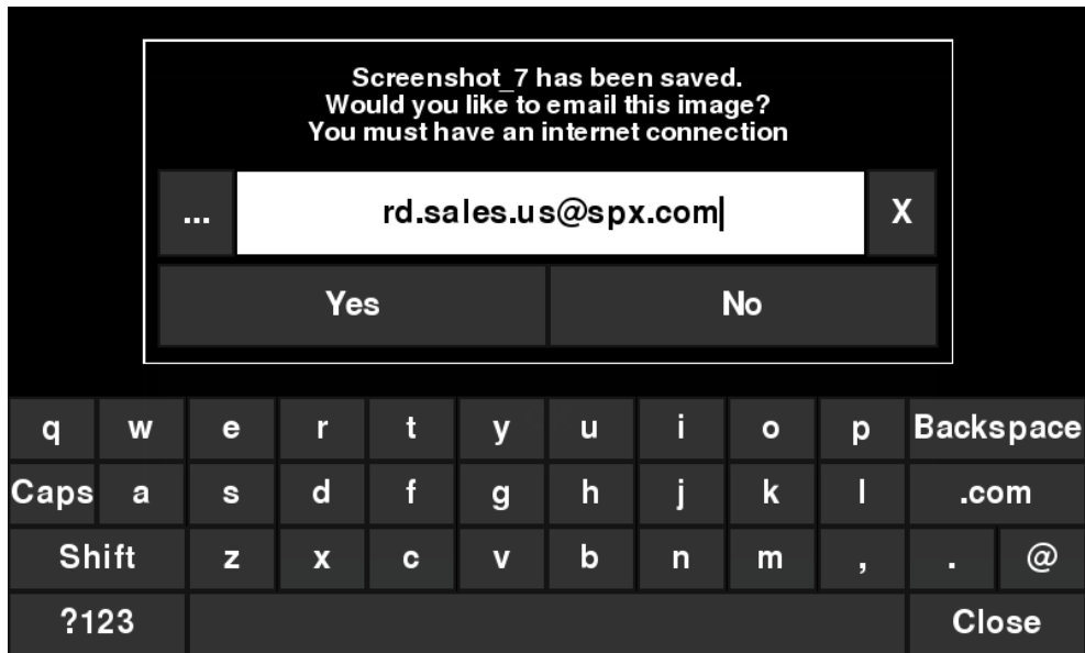
Figure 7-2: Message after pressing the Camera button on the Display Unit to capture the screen with WiFi enabled and a connection to a wireless network. The user can enter an email address to send the mini-report to
