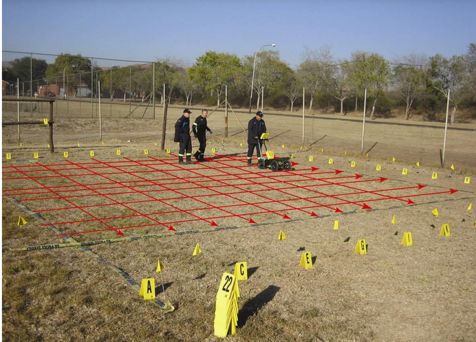
Figure 9-2: Example of a grid survey. The red lines are superimposed just to illustrate the concepts.
