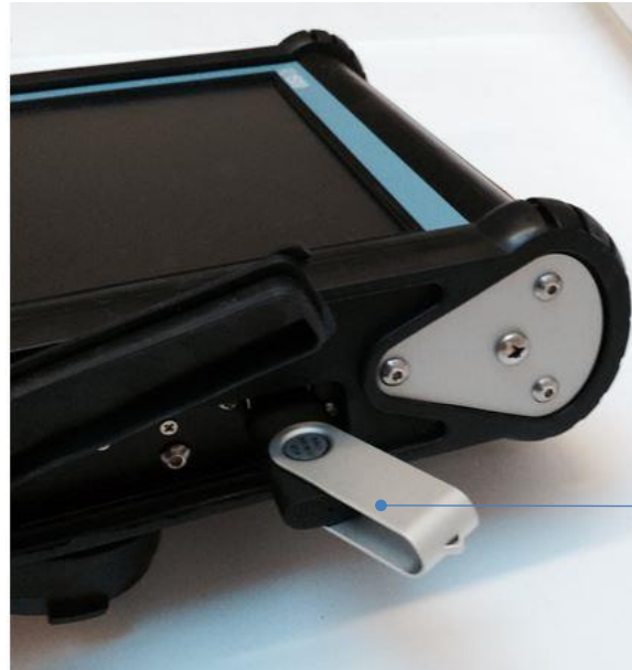
Figure 13-1: Insert a USB memory stick into the USB port on the Display Unit to export data.
