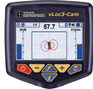
When directly over the sonde the arrow turns into a sonde icon
