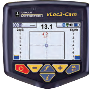
Directional arrows point to the sonde location
