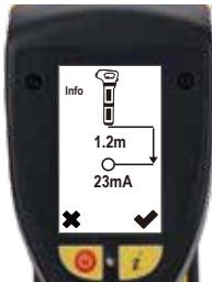
Press the *i* button for a depth reading with current measurement and logging options.
